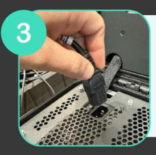
Connect the power supply to an electrical socket
