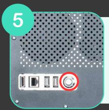
Press the power button on the front of the case (the button lights up when the computer starts)
